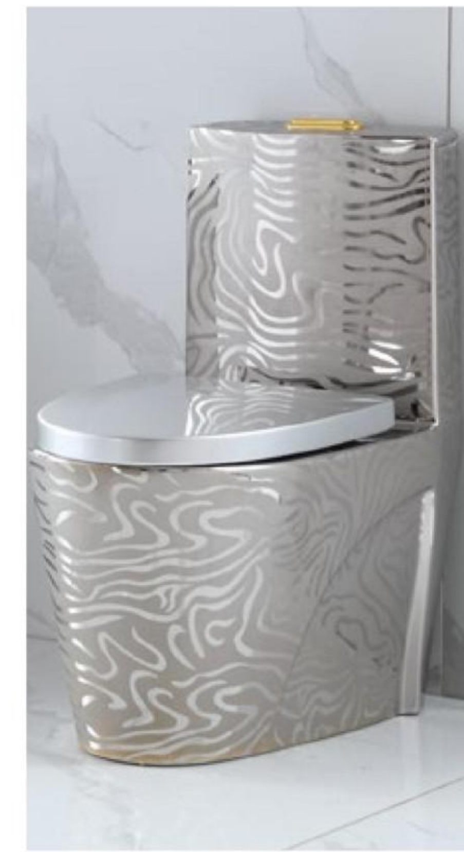
HS-AJ168 Washdown/Siphonic one-piece toilet 直冲/虹吸式连体坐便器 Size: 700*390*780mm P-trap: 180mm Roughing-in S-trap: 250, 300, 400mm Roughing-in
