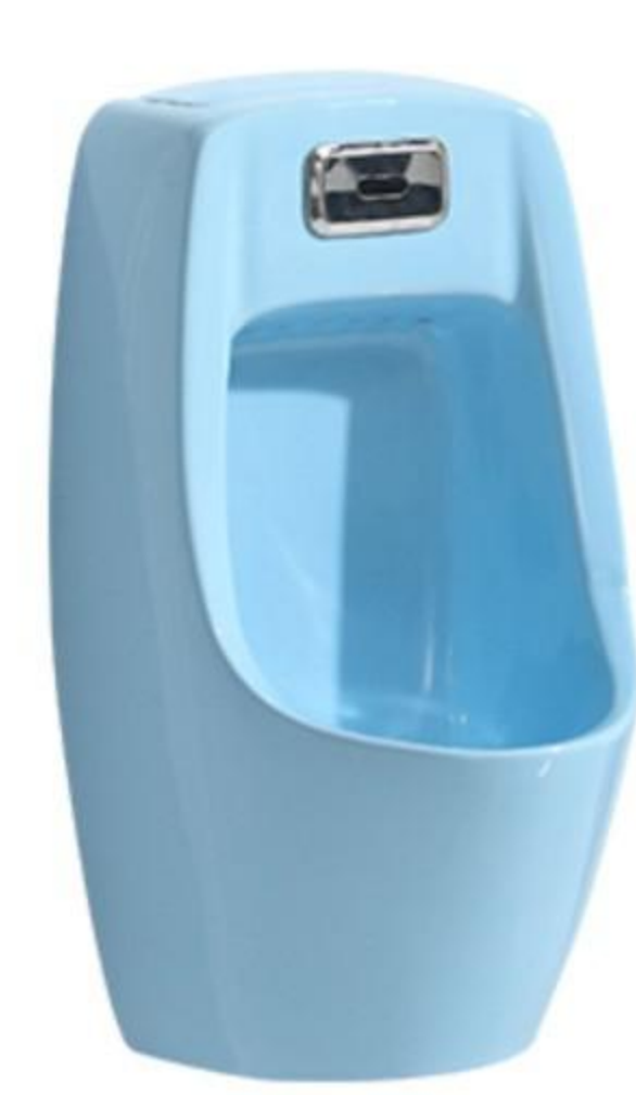
HS-006(儿童彩色小便斗) Wall-hung urinal Size:285*240*500mm 排污口中心离墙:80mm 排污口中心离地:80mm
