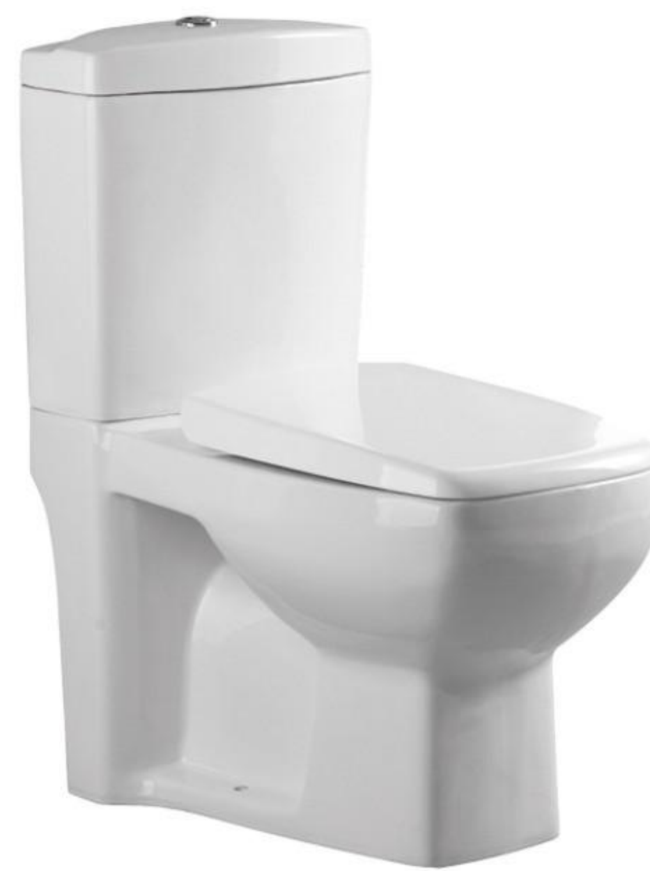
HS-TMS-2591 Washdown two-piece toilet Size:625*370*880mm S-trap,150-250mm Roughing-in P-trap,180mm Roughing-in
