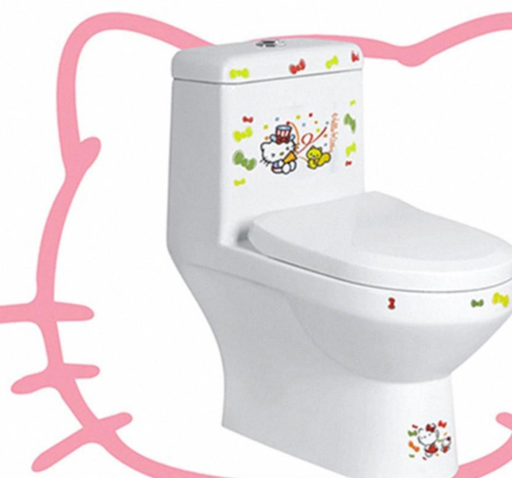
HS-2211K(儿童直冲连体座便器) Washdown one-piece children toilet Size:500*280*540mm 排污口中心离墙: 170mm 排污口中心离地: 140mm
