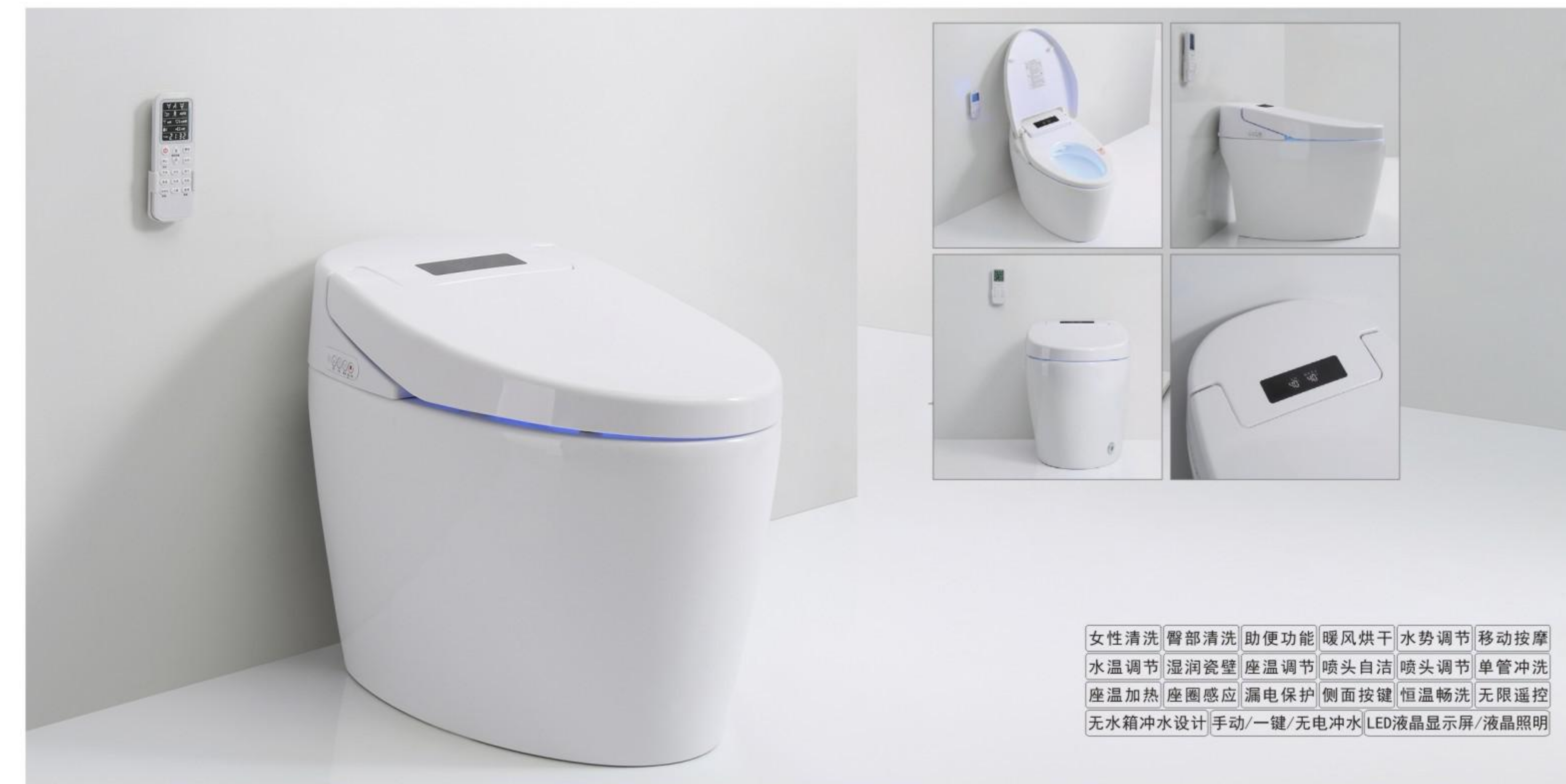
HS-ZA666 智能坐便器 Intelligent toilet Size:680*420*520mm S-trap,300.400mm Roughing-in 地排,排污口离墙300.400mm 无水箱即热式
