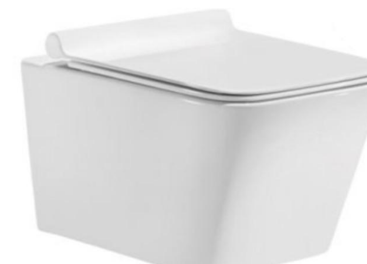
HS-804T Washdown wall-hung toilet Size:520*360*350mm P-trap,180mm Roughing-in
