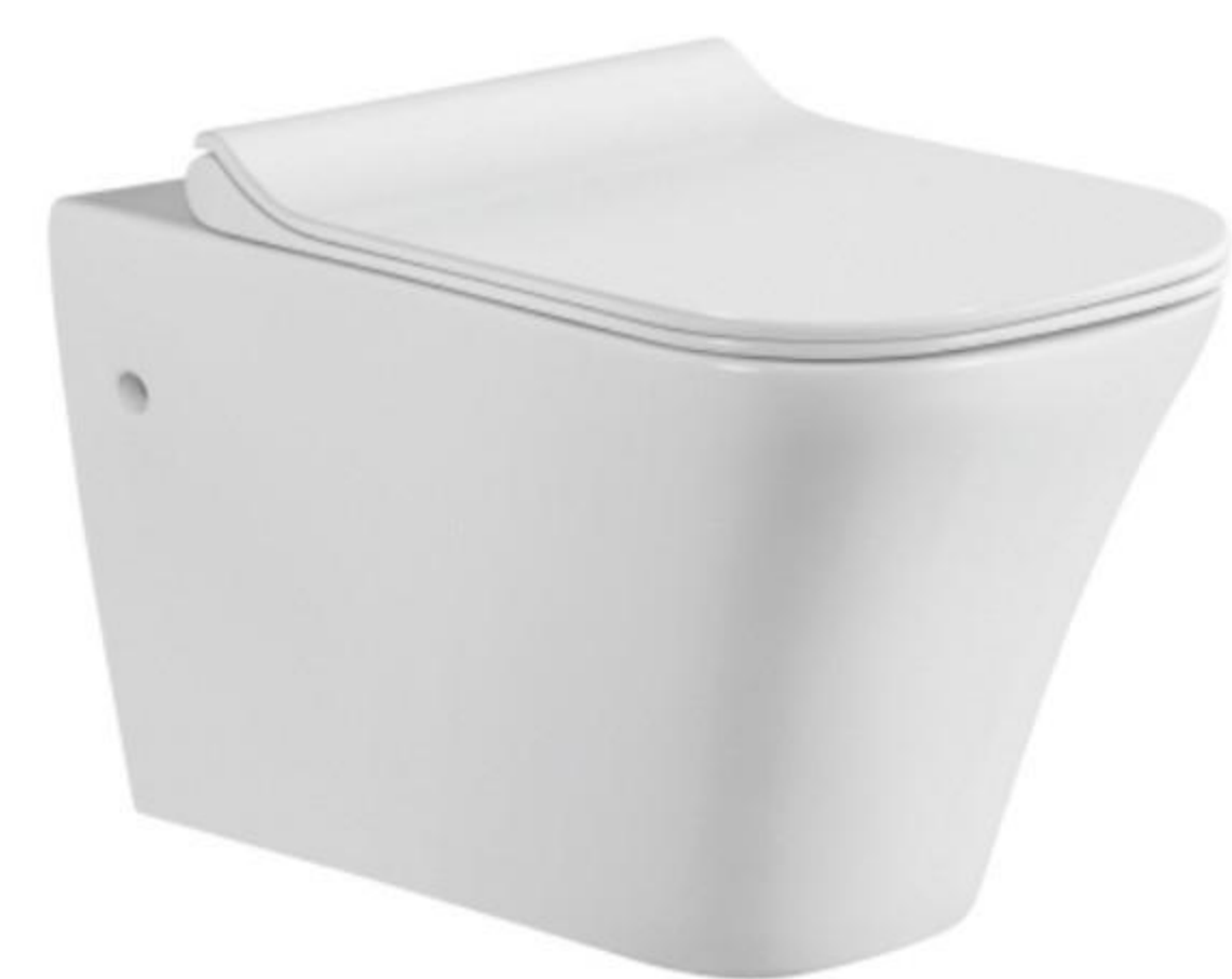
HS-F116 Washdown wall-hung toilet Size:560*350*340mm P-trap,180mm Roughing-in
