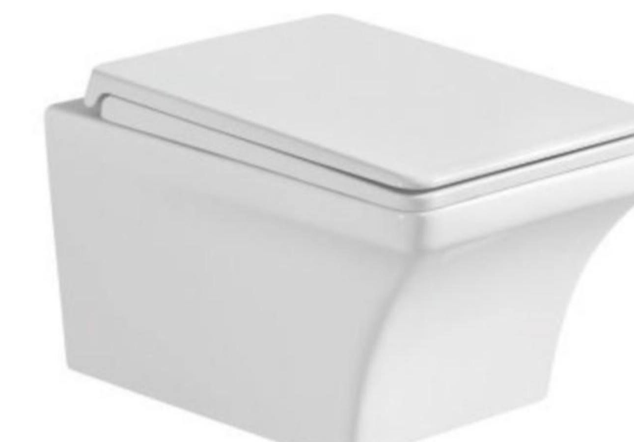
HS-801T Washdown wall-hung toilet Size:530*360*330mm P-trap,180mm Roughing-in
