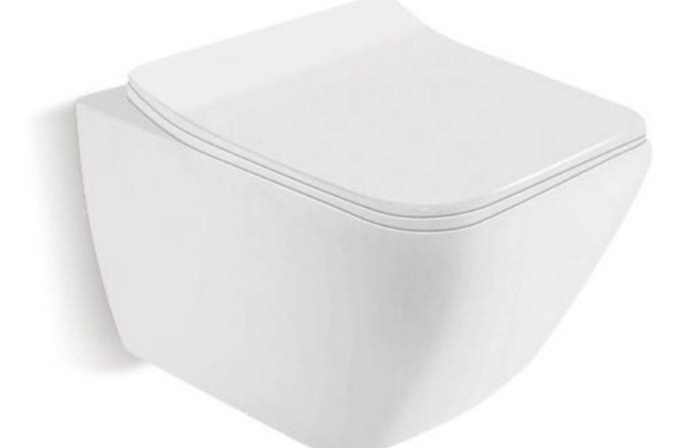
HS-8013D Washdown wall-hung toilet Size:530*365*320mm P-trap,180mm Roughing-in
