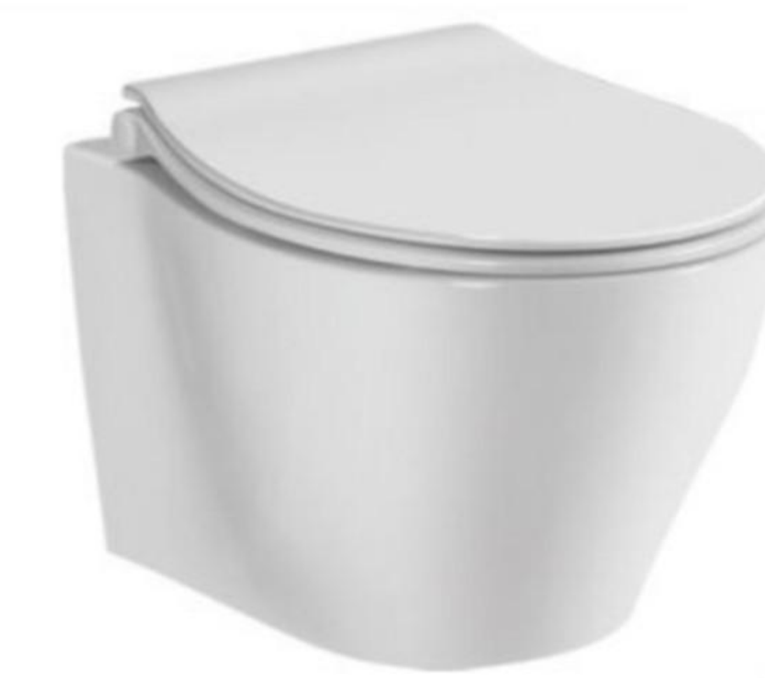
HS-803T Washdown wall-hung toilet Size:520*360*370mm P-trap,180mm Roughing-in
