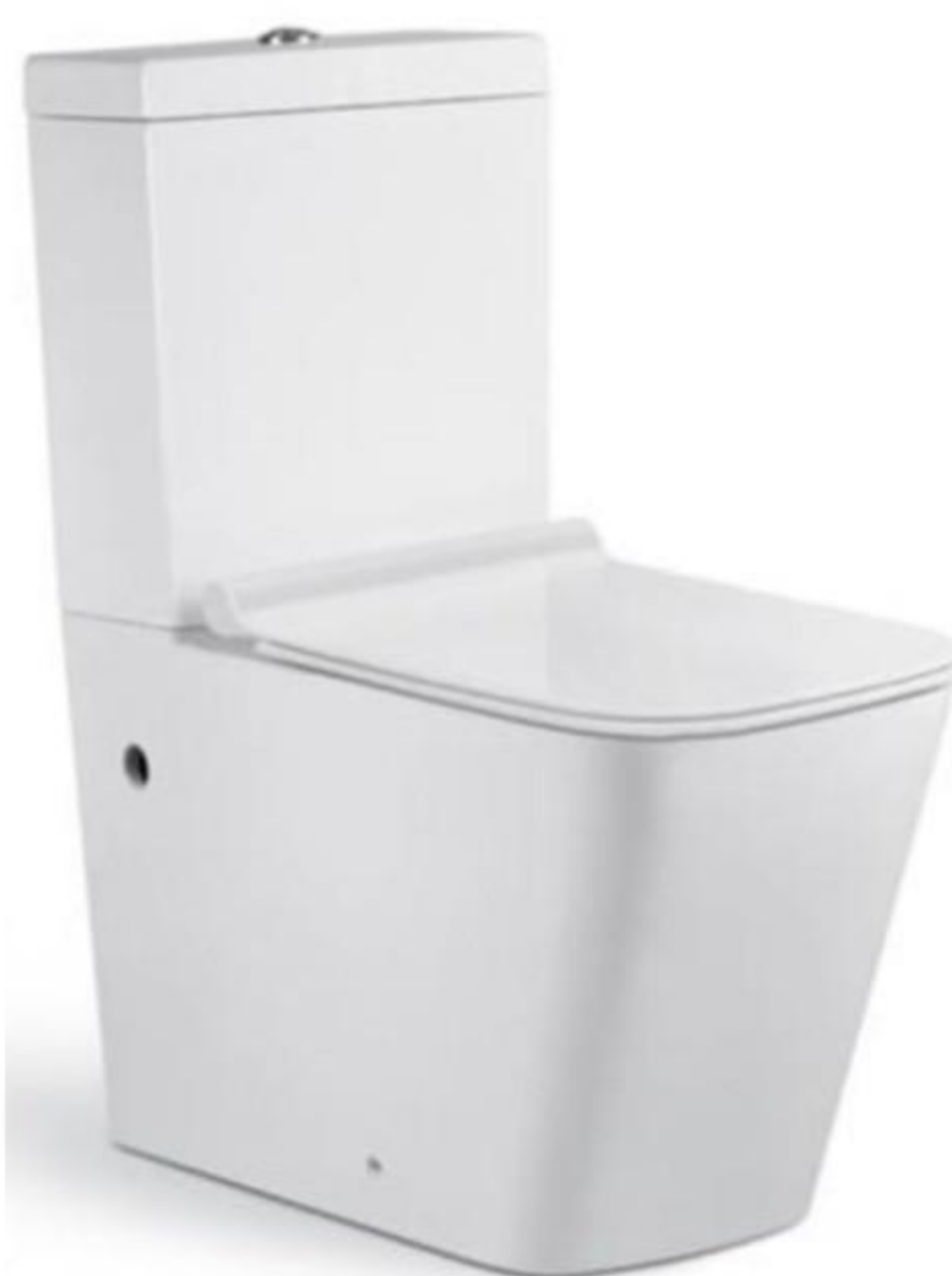
HS-9014AT Washdown two-piece toilet Size:720*390*765mm S-trap,250.300mm Roughing-in P-trap,180mm Roughing-in
