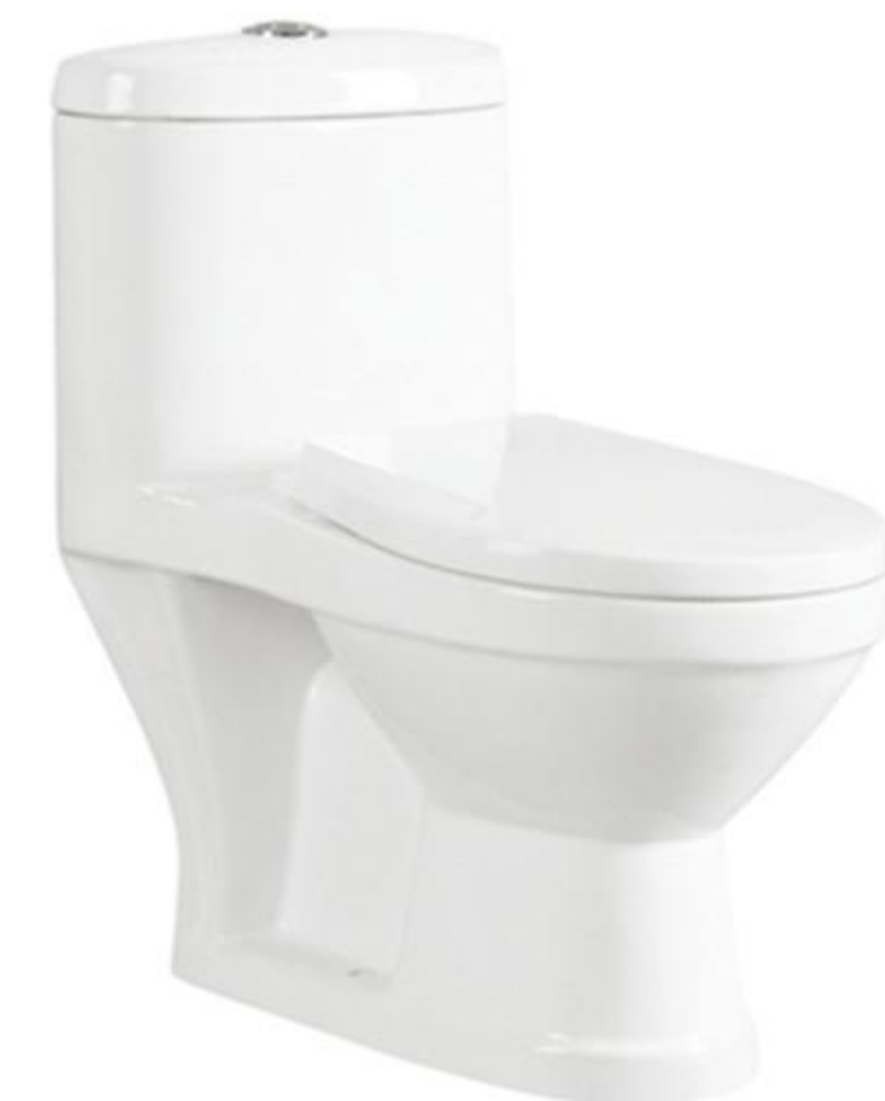
HS-2210白色(儿童直冲连体座便器) Washdown one-piece children toilet Size:500*285*530mm 排污口中心离墙: 200/300mm 排污口中心离地: 110mm
