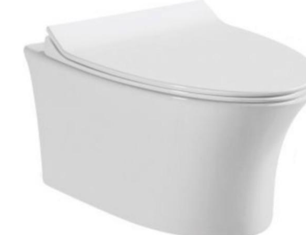
HS-802T Washdown wall-hung toilet Size:545*385*340mm P-trap,180mm Roughing-in
