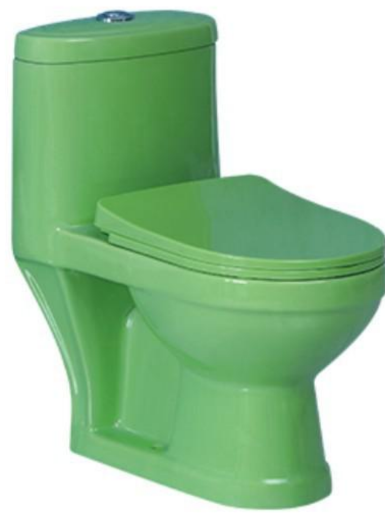
HS-2210(儿童直冲连体座便器) Washdown one-piece children toilet Size:500*285*530mm 排污口中心离墙: 200/300mm 排污口中心离地: 110mm
